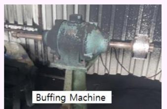
Presently, on the buffing machine, the buffing of the old tyres is done manually using 5HP motor.
